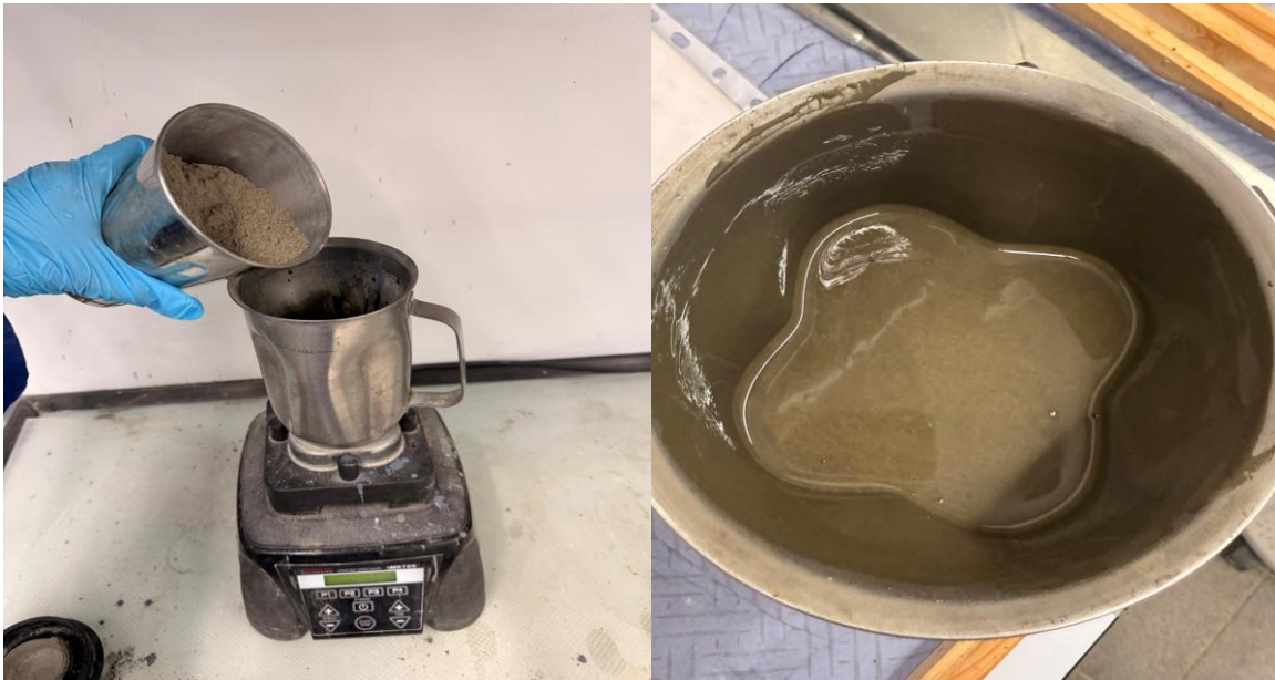
Figure 9: Slurry mixing step used for cement-sample preparation, based on standard well-cement laboratory testing procedures [2].
