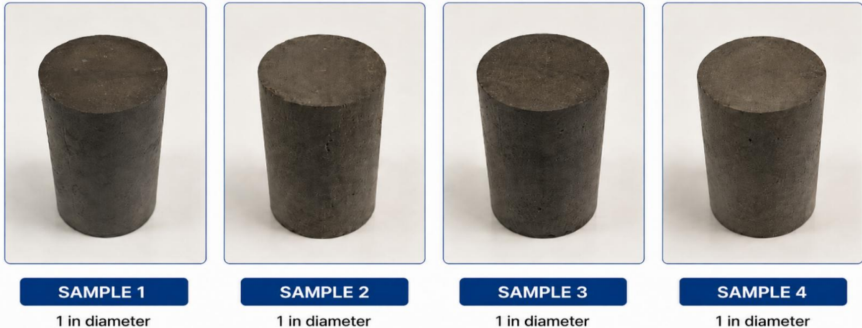
Figure 13: Post-curing cement samples prepared for baseline characterization and subsequent CO 2 -exposure testing.
