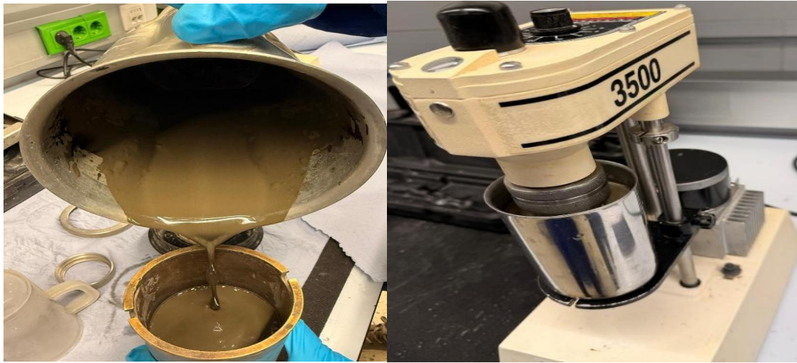
Figure 10: Conditioning slurry and rheology measurement, based on standard well-cement laboratory testing procedures [2].
