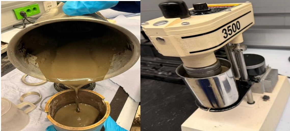
Figure 9: Conditioning slurry and rheology measurement
