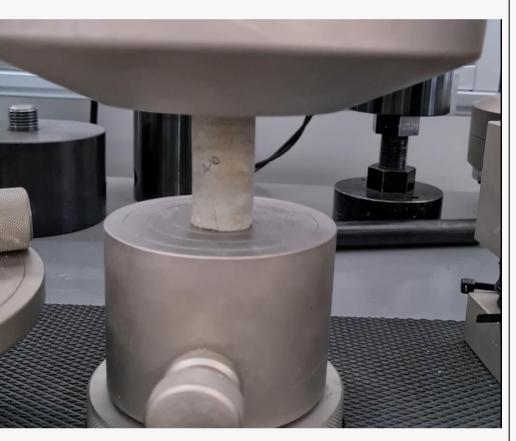
\*Note that for a valid test L/d should always be  $\geq 1.5 <$
