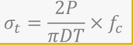
**P**: Maximal Stress  $\sigma_t$ : Tensile strength **D**: Sample Diameter fc: correction factor **T**: Sample Thickness (equal to that of platen)
