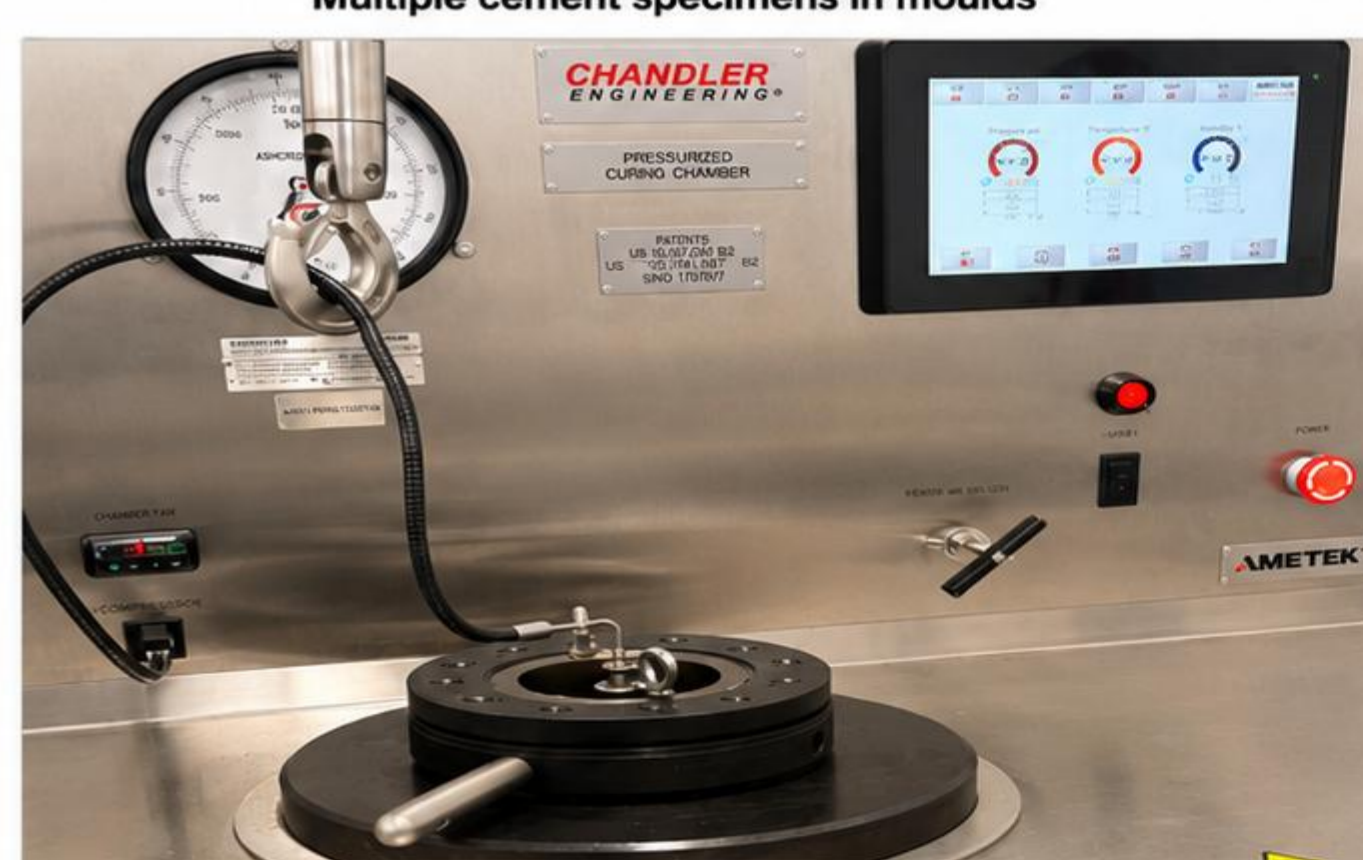
Pressurized curing chamber
