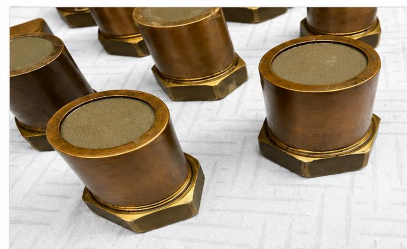
Close-up of cured cement specimens
